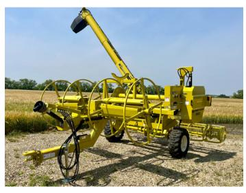
bag is lifted and pulled onto the drive spools, it is gently guided into place by the RENN roller and hold down system – reducing stress on the bag and helping prevent spillage. RENN's continuous-flow unloading system effortlessly draws the Unloader and power unit into the bag, while quickly unloading the bag contents through high-capacity discharge augers.
