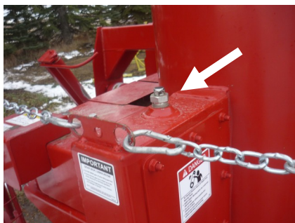
Fill Access - 0.5 liters when Empty or runs out level check
