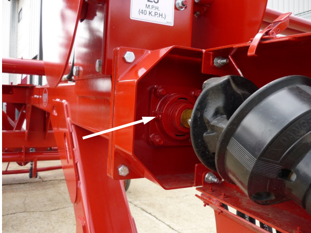
Primary Driveline Flange Bearing
