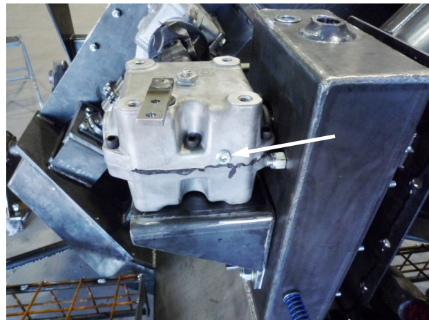
90° Gearbox Level Check
