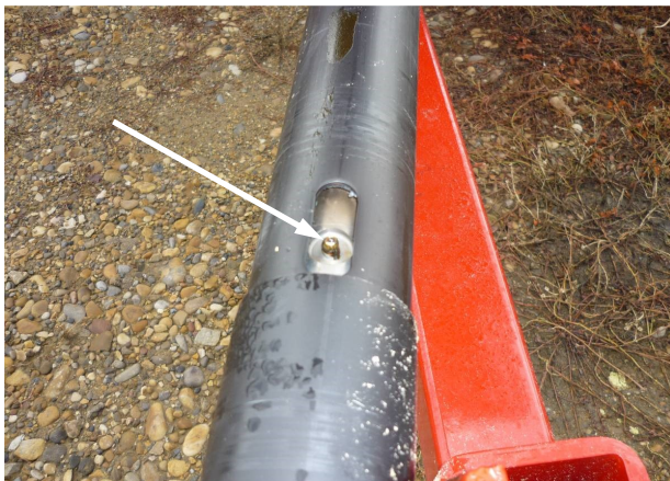
PTO, mid grease zerk, extend PTO and rotate shield to find zerk (every 8 hours)
