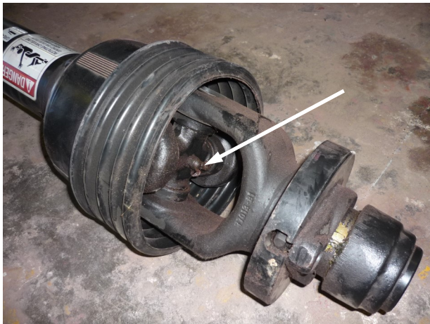
PTO, front and rear yoke: grease zerk (every 8 hours)
