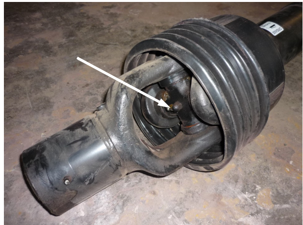
PTO, front and rear yoke: grease zerk (every 8 hours)
