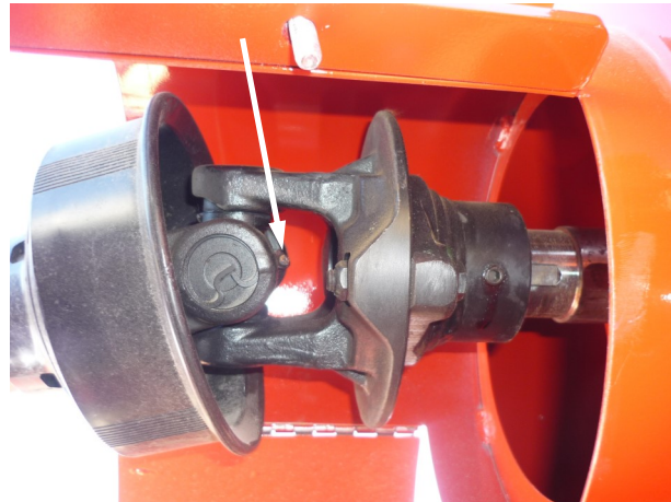
Main shaft bearings: grease zerk front and rear (every 50 hours)
