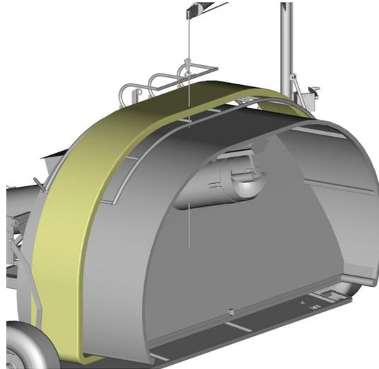
10. Raise the bag lift further to eliminate any creases or bunches of folded bag in the bag pan region. This will eliminate plastic bunched under the bag. Do not overload the bag crane and watch for any downward deflection of the horizontal arm.
