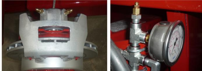
Auger, end bearing set, sealed units; torque clamp bolts; check bearing seal on outer bearing and set collar tight and set screw locked
