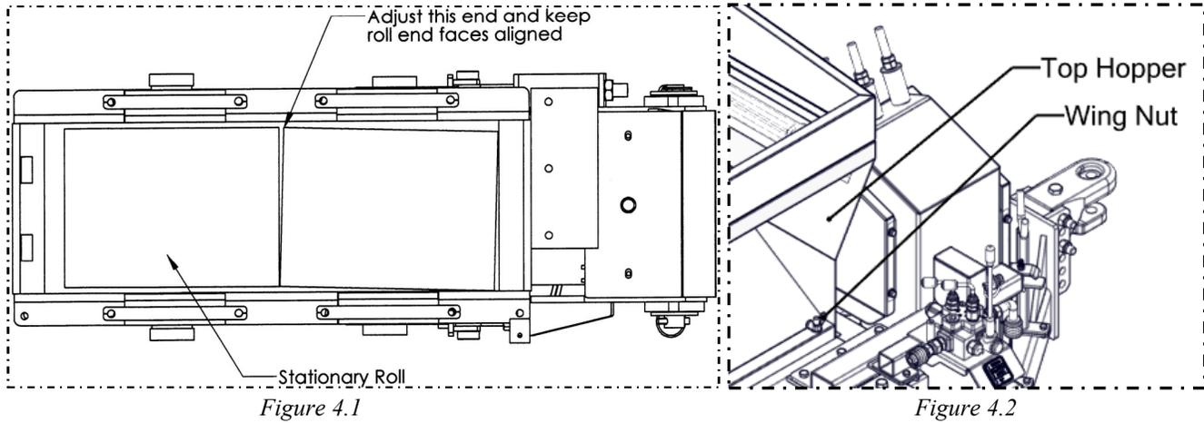
Loosen the wing nuts holding down the top hopper (Figure 4.2) and tip it over center, rotating on the hinge pin until it hits the stoppers.
