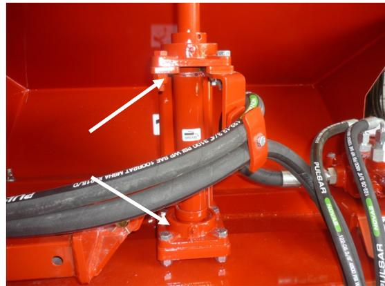
For discharge gearbox oil level check -
