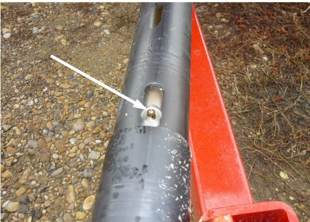
Main bearings: grease zerk front and rear (every 8 hours)
