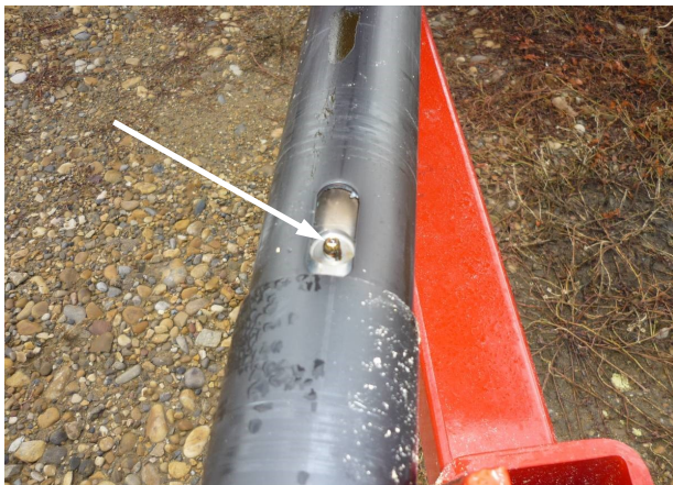
PTO, mid: grease zerk, extend PTO and rotate shield to find zerk (every 8 hours)
