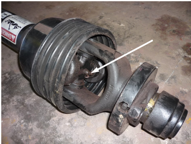
PTO, mid: grease zerk, extend PTO and rotate shield to find zerk (every 8 hours)
