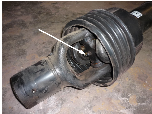
Main bearings: grease zerk front and rear (every 8 hours)
