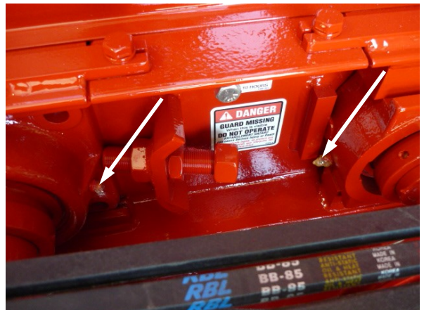
Main bearings: grease zerk front and rear (every 8 hours)
